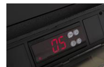
0 - 10 degrees electronic temperature control
