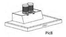
10. See pic 10, Put the chimney on the cooker hoodand be sure that the inside chimney can be adjusted the height in it freely. Then lead the expansion pipe to outside.
