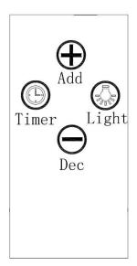
1. press button once , the light is on, press again, the light is off. The lighting button it is controlled separately and will not affect any other functions.
